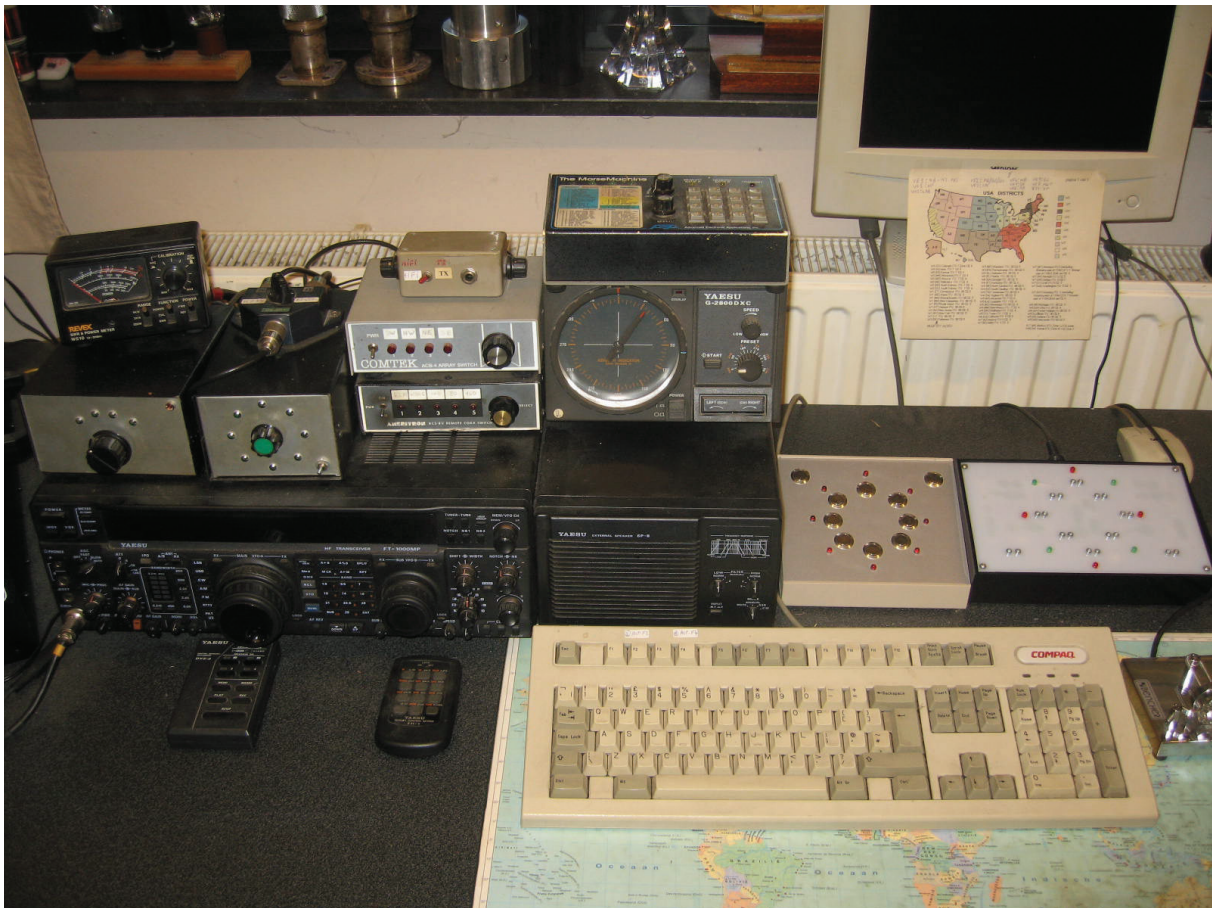
Figure 9 - Overview of the different switchboxes. On top (middle) of the 1000mp radio is the old rotary switch version (left to that is the homebrew K9AY controlbox). Right hand side of the speaker, the two new versions: first the push button version, followed by the touch button switchbox.
