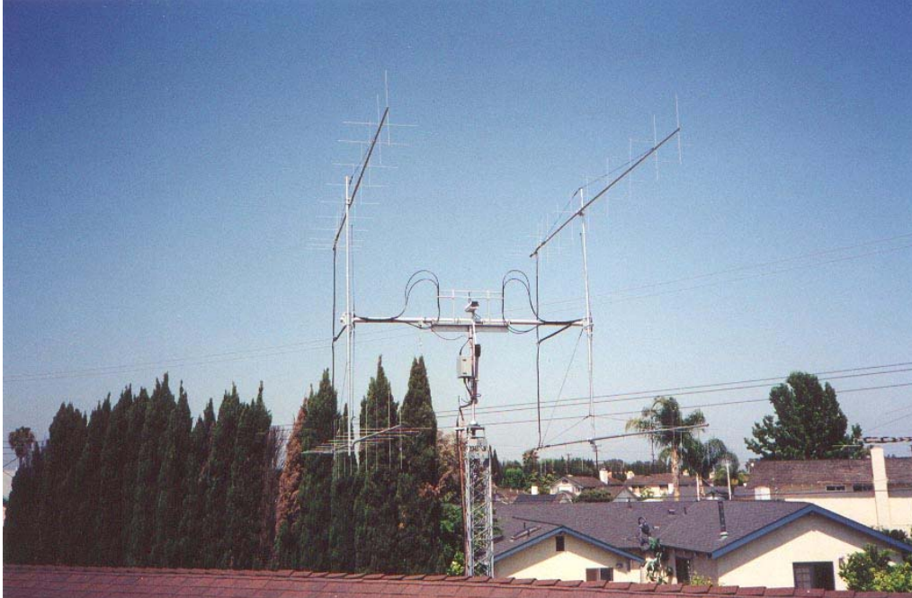
Photo B – EME array at K6PF consisting of four x-pol yagis with a mast mounted preamp and relays and TV camera
