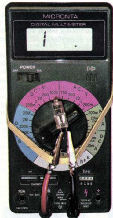
Figure 2—The proof that the filament is broken. The "1" on the DMM display indicates an overflow (infinite resistance).
